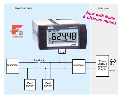
The BA448CF-F Fieldbus Indicator is an intrinsically safe instrument that can display up to eight fieldbus process variables within a hazardous area. A numeric annunciator on the left hand side of the screen shows which variable is being displayed. This version of the instrument supports FOUNDATION ™ fieldbus protocol; for PROFIBUS PA systems an alternative version is available − please see the BA448CF-P PROFIBUS datasheet.
